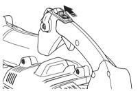
**CAUTION!** The stop switch automatically returns to the start position. In order to prevent unintentional starting, the spark plug cap must be removed from the spark plug when assembling, checking and/or performing maintenance.
