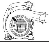
WARNING! Never use the blower if the screen is not in place. Before use, check that the screen is in place and undamaged.
