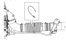
Connect the straight pipe and pipe end. Push the pipes together and turn them so they lock.
