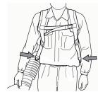
Tighten and adjust the breast belt for the best working position.
