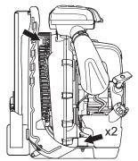
Check that the vibration damping element is undamaged and securely attached.
