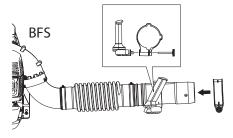
Adjust the position and angle to achieve a comfortable working position, and tighten.  Use the clamp to fasten the cabling to the flexible hose. (BTS)
