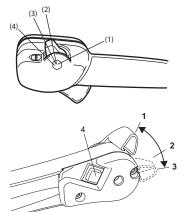
It is not allowed to set the stop switch in full throttle position.
