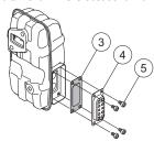
To remove the spark arrestor screen proceed as follows:
